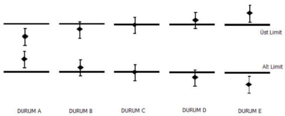
**State A:** The measurement result is within limits (below the upper limit or above the lower limit) even when expanded by uncertainty. In this case the product **meets** the specification.
